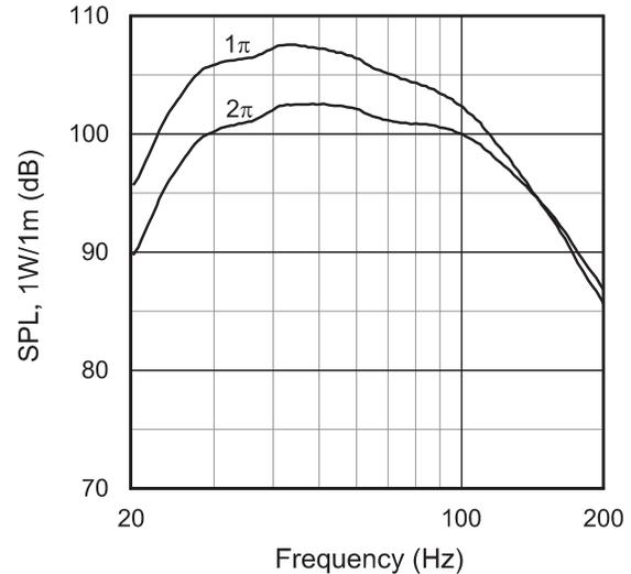
4642A frequency response, 1 watt at 1 meter, with 150 Hz Linkwitz-Riley 4th order low-pass filter and 2nd order high-pass filter at 25 Hz with  $Q=2$ .  $1\pi$  (upper curve) and  $2\pi$  (lower curve) conditions.
