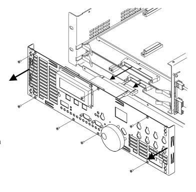
7. Remove the Cat. No. 794 upgrade kit board from its anti-static bag and plug it into the **left-hand** side of the main board by aligning the two connectors shown in the figure. Press down on each side making sure the connectors are fully seated. The board can be oriented only one way for the connectors to match.
