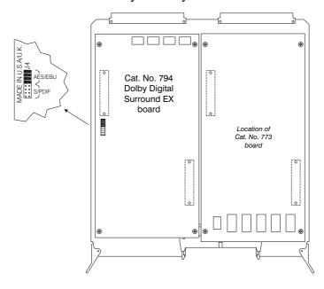
**Note:** The Cat. No. 794 will not function if it is installed in the right-hand location. This area is reserved for the Cat. No. 773 Dolby Digital decoder board.
